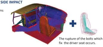
The accelerations (in the three directions) registered during the crash test nearby the driver seat are imposed to the master node.
